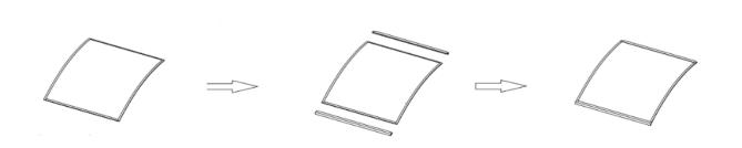
Insert aluminium bars on the two short sides.
