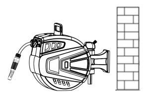
Fasten mount seat to the wall with screw.
