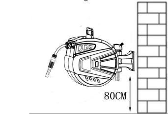
It is recommended to install the mount seat 0.8 metre from the mount seat to floor.
